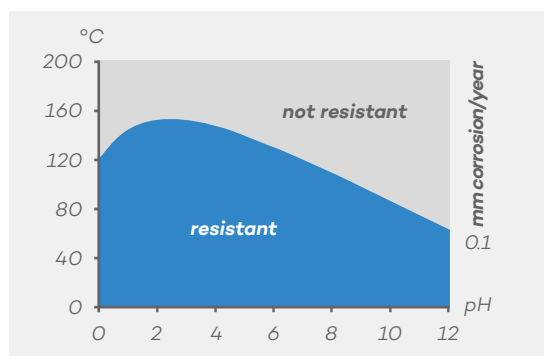
Isocorrosion curve of pH enamel
